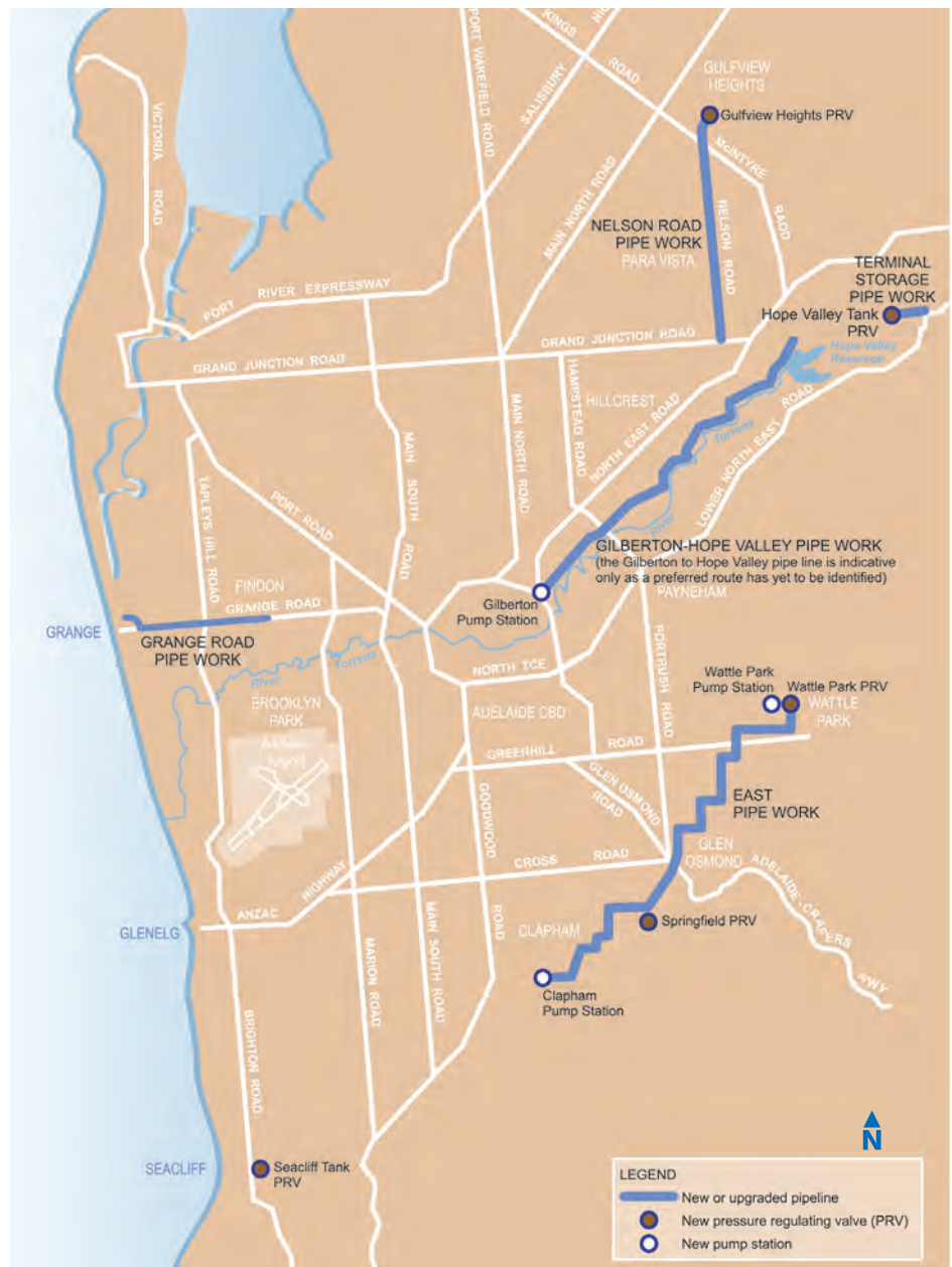
An overview of the elements of the North-South Interconnection System Project to connect northern and southern portions of Adelaide's water supply network.
